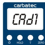
3. With the "1" flashing, rotate the box clockwise, 90° and press the "ZERO" button. The screen will display "CA2". Don't move the device until the "2" begins to flash.
