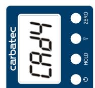
6. Turn the box clockwise, the final 90°, until it sits upright as at the start. Press the "ZERO" button. The screen will display "CA5". After 3 seconds without movement, the display will return to 0.00, and the calibration will be complete.
