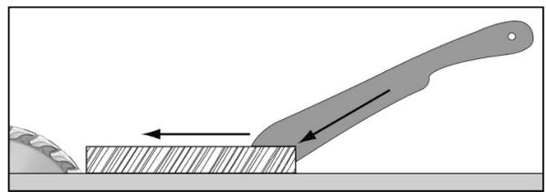
Feeding: Place the notched end of the push stick against the end of the workpiece, and move the
