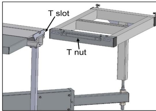
4. Insert the shaft under the cross cut fence into the hole of the cross cut table, and adjust the fence's position front and back. The fence could be located in the forward or rear position.
