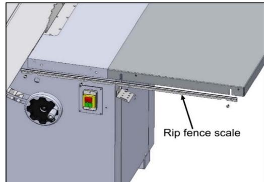
2. Fasten the rip fence rail to the table by screws on the rail.
