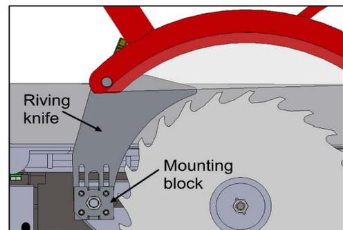
The riving knife also prevents the freshly cut sides of the workpiece from pinching the blade and causing kickback. For maximum effectiveness of this safety design, the riving knife must be positioned within 3–8mm from the blade.
