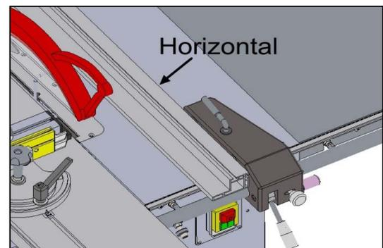
4. Slide leading end of rip fence so it is even with center of main saw blade
