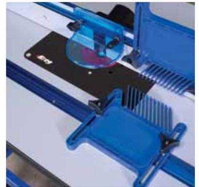
Wedge-lock hardware allows the featherboards to be separated and used in two ways: mitre slot or T-slot.
