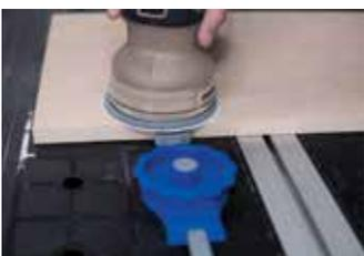
Low-profile design keeps clamp out of the way while working.
