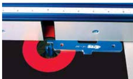
Step on the end of each setup bar precisely sets fence offset distances on the router table or table saw.
