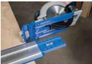
A Starting Block in the Accu-Cut™ track aligns and supports your saw to ensure that you can start every cut accurately. Plus, the Starting Block allows normal blade-guard operation to ensure safety as you start each cut, and helps guide the saw cord while cutting.
