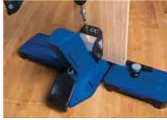
Multi-featured jig for creating pocket-hole joints in materials from 13 mm to 38 mm thick
