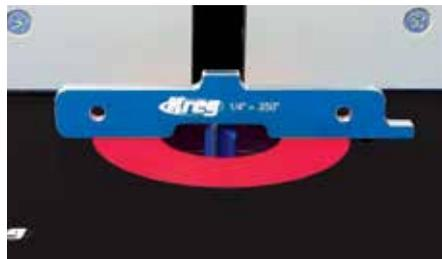
Concave step on the bottom of each setup bar straddles router bit or saw blade for precise height adjustment.
