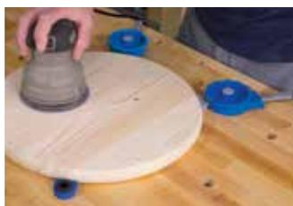
Clamp shoe holds flat and rounded shapes, as well as 90°.
