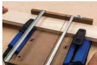
A kerf line you cut into the MDF base shows exactly where your saw will cut.
