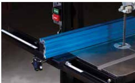
The aluminium fence is incredibly strong, straight, and built to last for years. The face and top edge of the fence contain T-slots for adding stops, resaw guides, and more.
