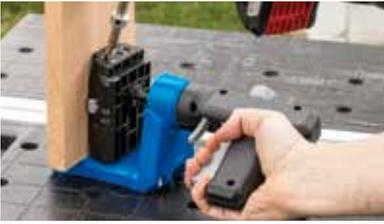
Versatile jig for creating pocket-hole joints in materials from 13 to 38 mm thick
