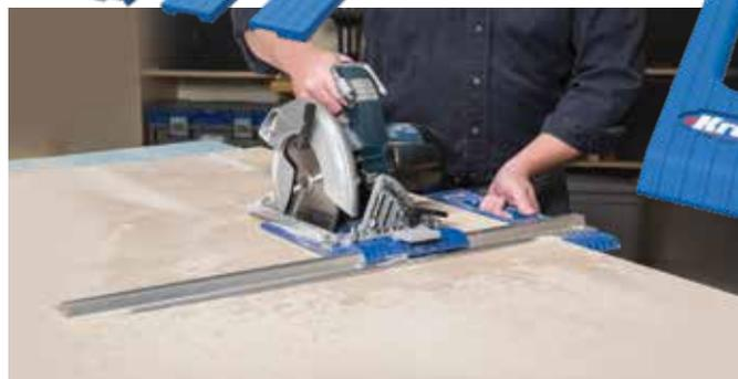
No measuring or marking required thanks to a built-in measuring scale and precision cursor. Just lock in your cut size, and go.
