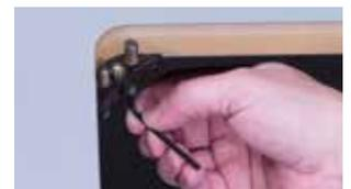
Two adjustable set screws on each Leveler make it easy to set the router plate flush with the table surface.
