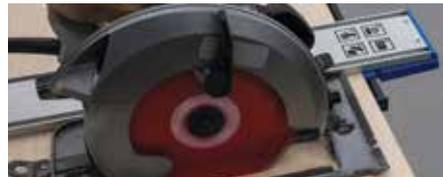
Works with left- and right-blade circular saws, as well as jigsaws and trim routers
