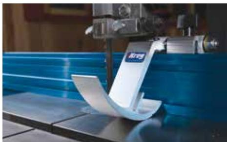
Add an optional Swing Stop™ or a Production Stop to the fence to simplify making accurate, repeatable cuts to a set depth, such as when cutting tenons (See page 24).
