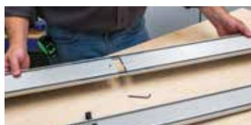
Aluminium guide rail leads cuts precisely along a straight line
