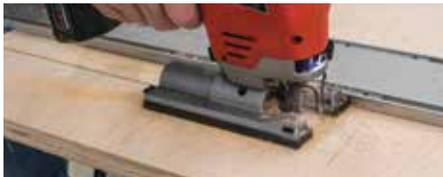
Aluminium guide rail leads cuts precisely along a straight line
