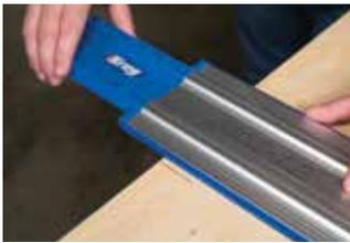
Eliminate the guesswork by simply aligning the track with your reference marks. Guide Strips on each edge of the Accu-Cut™ show you exactly where your saw will cut, so you can make every cut with confidence.
