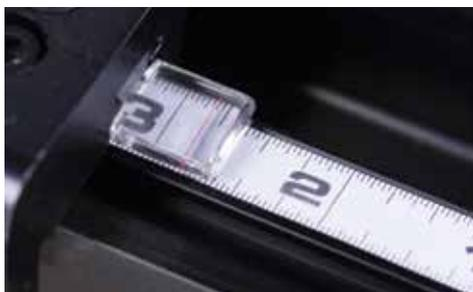
Magnified and easy-to-read for even the smallest adjustments, the Precision Lens Cursor lets you accurately set up the fence for cutting veneer, tenons, and more.
