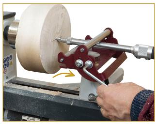
Slacken the cantilever locking screws and adjust the upper roller until it sits securely on the top of the tool shaft and lock into position
