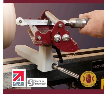
The Robert Sorby SteadyPRO is a very easy to use jig that gives additional tool support when bowl turning, hollowing and when doing spindle work.
