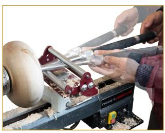
The rollers allow the tool to move smoothly, whilst being held securely
