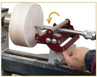
Place the desired tool onto the lower roller and adjust the height of the stem in the banjo, so that the cutting edge of the tool is at the required position and lock the stem into place
